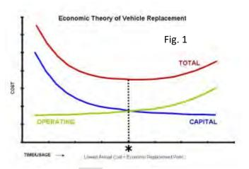
The total cost curve is different for every type of vehicle and, indeed, for every individual vehicle of a given type. This variability is caused by differences in the design and engineering of different types of vehicles / equipment, in operating environments, in the quality-of-care vehicles / equipment receives, and a variety of other factors.
