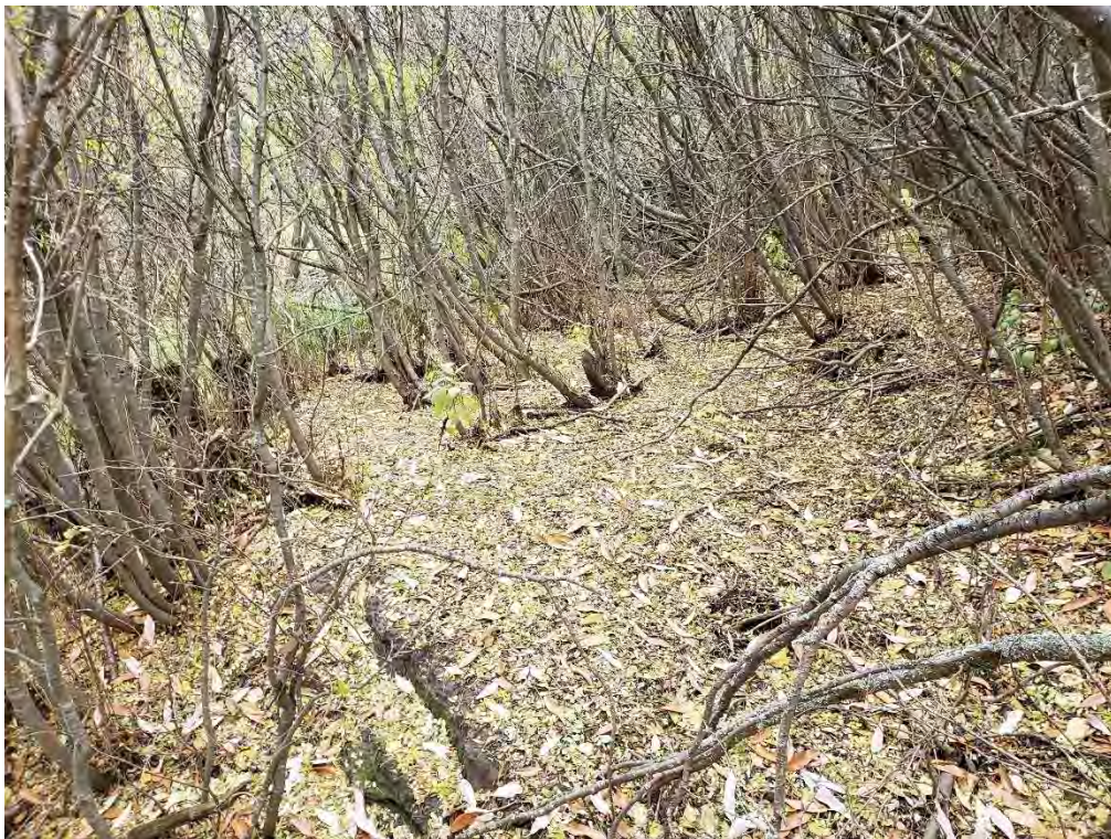
Photo 4 – Slope below Old Firehall Building. Willows showing curvature near base from slope creep.
