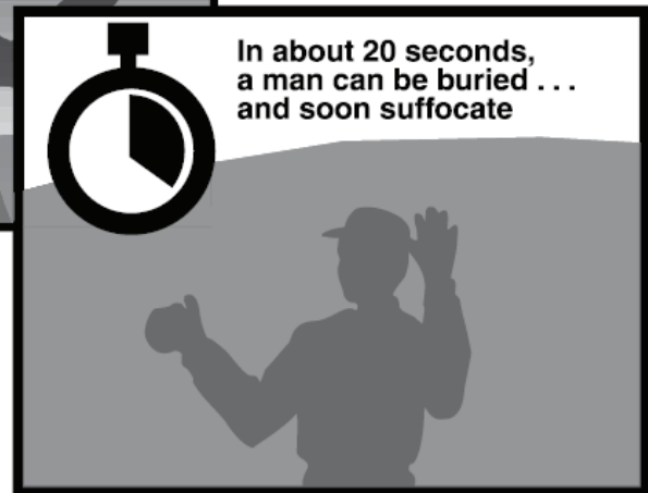
Figure 3. Flowing grain can exert a tremendous pull on a body caught in the flow. You will be helpless within three to four seconds. In 20 seconds or less, you can be completely buried.
