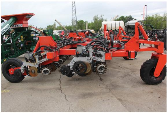
Future production PPS models will get heavier castor wheel assemblies and sturdier wing fold designs. The changes are based on the field performance of this and two other working prototypes. photo: Scott Garvey
