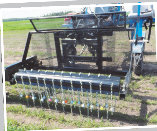
Hail Simulator mounted on SARDA's spider sprayer.
