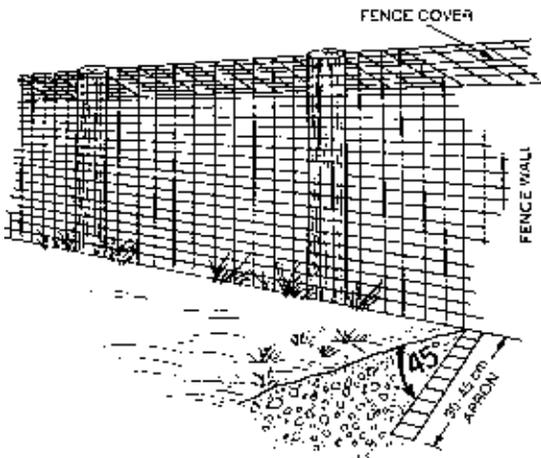
Figure 2. Angle apron fence (cover with dirt).
