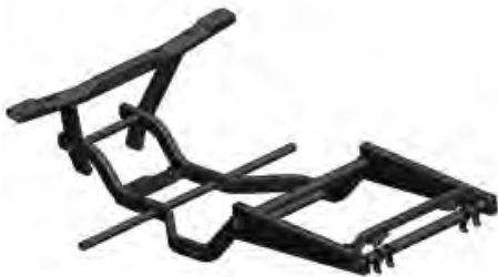
XUV two-passenger mainframe structure – rear-left view
