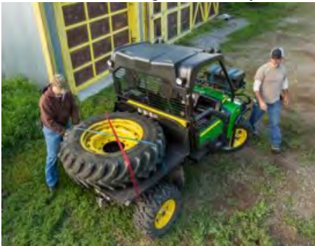
Deluxe cargo box converted to a flat bed (XUV 825 shown)
