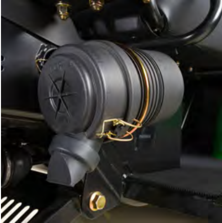
Battery location and remote air intake canister shown on XUV825
