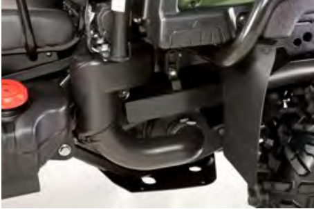
Side view of CVT intake and clutch on closure (XUV855 shown)
