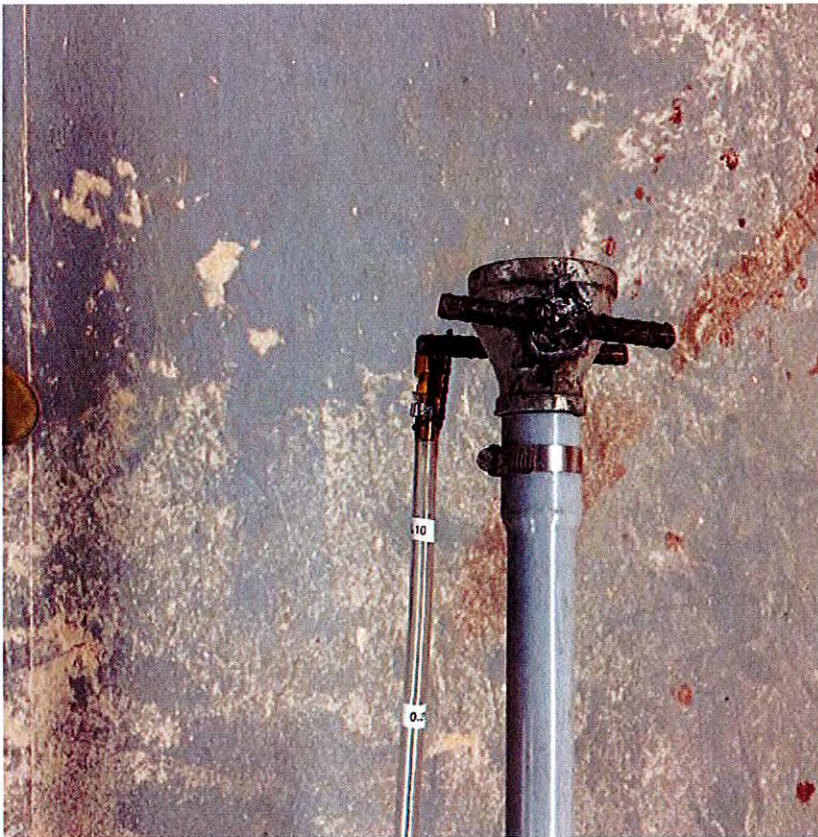
Example of how clear tubing would fit inside of protective sleeve casing
